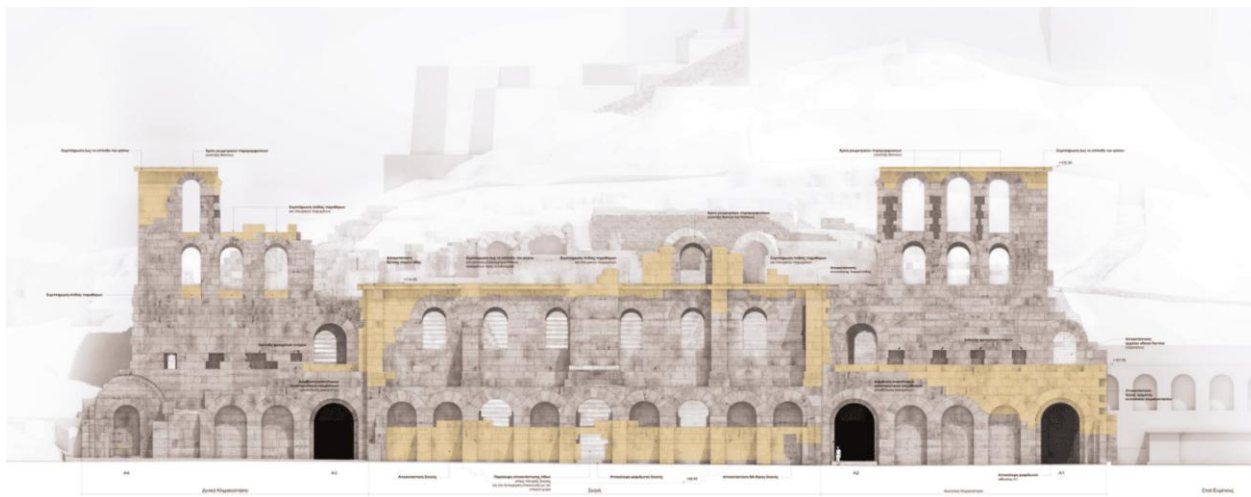
FIG. 5a. The south front of the Odeion of Herod Atticus, after the projected reconstruction. Reconstructed parts indicated in yellow. Source: LIFO, 23.2.2026
