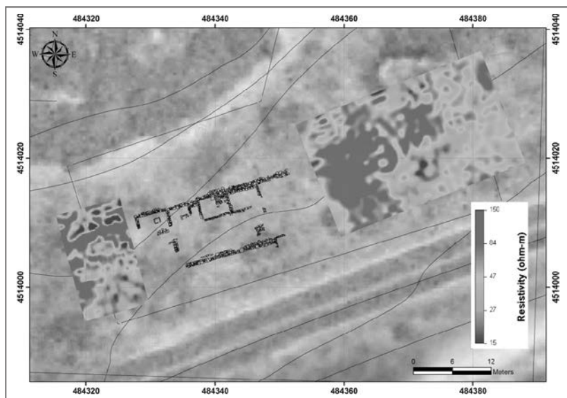
Fig.2: Resistivity distribution (slice) at the depth of about 1.0 m in ancient Argilos (Bonias et al., 2018). This result has been obtained by slicing the volume of the 3D resistivity distribution which was yielded by 3D data inversion.
